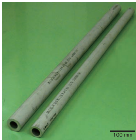
図9 USC141のボイラーチューブ試作材の外観 Fig. 9 Appearance of USC141 trial tube
