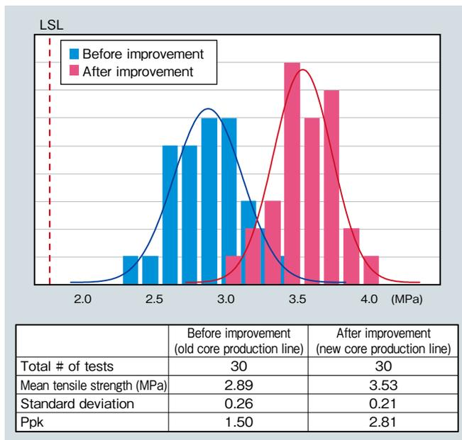
Fig. 6 Core tensile strength capability histogram comparison
