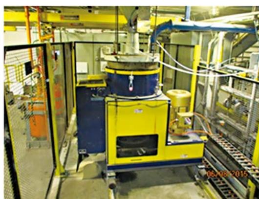
Fig. 5 Sand mixing system
