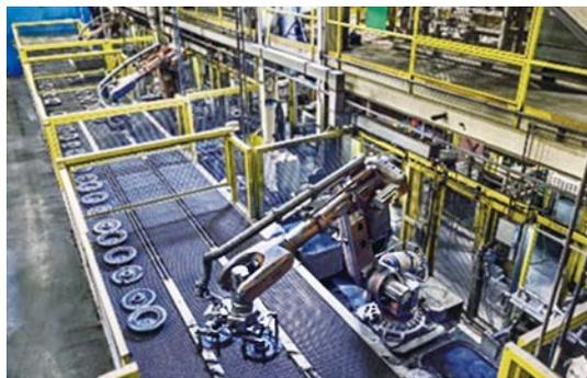
Fig. 2 Dual-station core machine with robot cell
