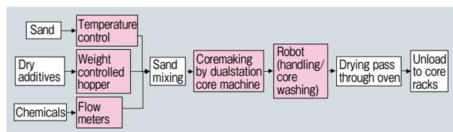
Fig. 1 Warm-box sand coremaking process
